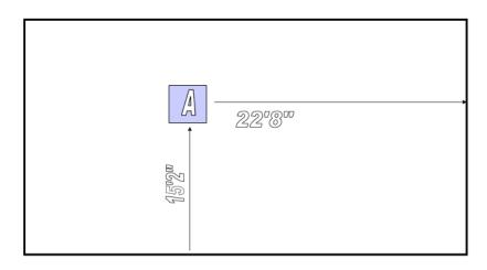
Figure C-5. Rectangular coordinate method of measurement
