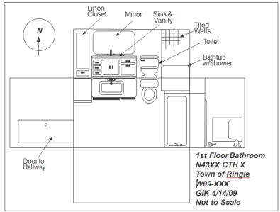
Figure C-2. Projection sketch of bathroom
