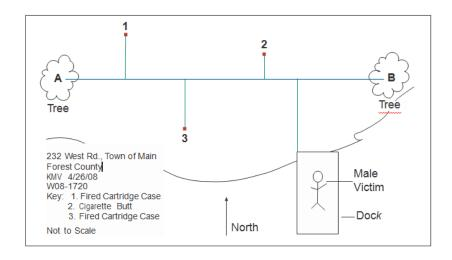
Figure C-6. Transecting baseline coordinate method of measurement
